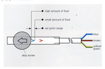
Color code of the electrical connections (normally open or normally closed operation)
